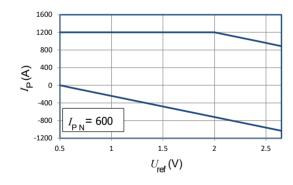
$$\begin{aligned} & \text{Upper limit: } I_{\text{p}} = 1200 \; (U_{\text{ref}} = 0.5 \; \dots \; 2.0 \; \text{V}) \\ & \text{Upper limit: } I_{\text{p}} = -480 \times U_{\text{ref}} + 2160 \; (U_{\text{ref}} = 2 \; \dots \; 2.65 \; \text{V}) \end{aligned}$$
